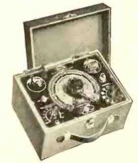
\* Resistance bridge and condenser analyzer for servicing. Improved type has direct reading scale and 6E5 visual balance indicator. Measures capacity 0.00001 to 70 mfd. resistance 50 to 2,000.000 ohms. Shows power factor of electrolytic condensers and insulation resistance up to 1,000 unegohms. Built-in power supply— 110 AC. Model CB-1-60—net \$19.20. Solar Mfg. Corp., 599 Broadway, New York City—RADIO TODAY
