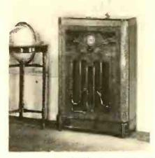
★ Three-band farm or summer cottage set for operation from storage battery. Seven tubes in superhet circuit—range, 540-1500, 1450-3500, 5600-18,000 kc. Full vision dial with dual-ratio vernier. Vibrator power unit—permo-dynamic speaker. Model 115. Stromberg-Carlson Telephone Mfg. Co., Rochester, N. Y.—RADIO TODAY
