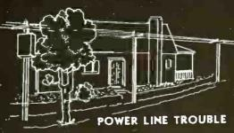
Leaky and dirty insulators Defective power transformers Bare wires contacting trees
