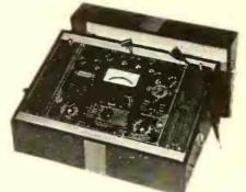
★ Latest Triplett tube tester checks tubes on basis of shorts and power output. Also tests electrolytic and paper condensers. Meter calibrated for AC-DC volts, DC milliamperes, decibels, and ohms. Furnished in either counter or portable models. Model 1501—list \$70, Triplett Electrical Instrument Co., 122 Main St., Bluffton, Ohio—RADIO TODAY
