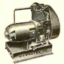
★ Portable power and light plant. Capacity of 300 watts at 110 volts 60 cycles AC. Generator is directly coupled to gas engine. Produces no radio interference—weighs 50 pounds. Katolight Jr.—list \$84. Other models (DC) available: 150 watts 6 volts—\$59.95; 200 watts 12 volts—\$62; 300 watts 32 volts-\$65; 300 watts 110 volts-\$69. Kato Engineering Co., Mankato, Minn.-RADIO TODAY
