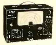
★ Test oscillator using fundamentals on all bands covering 60 to 60,000 kc Cast aluminum case with compartments for individual circuits—Faraday shield isolates instrument from AC lines. Has 6E5 tube for output indicator—modulated output at 400 cycles. Size  $10 \times 7 \times 4\frac{1}{2}$  weight 10 pounds. DayRad model 36-A—net \$36.75. Radio Products Co., 125 Sunrise Pl., Dayton, Ohio— RADIO TODAY
